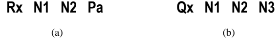
Fig. 6. A gene coding a resistor (a) and a bipolar transistor (b): Rx-loci is the resistor's name; Qx-loci is the transistor's name; N1, N2, N3 -loci are the nodes for the first, the second and the third pins; Pa-loci is the resistor's parameter.
