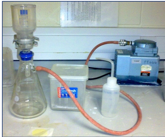
Figure 3-12. Vacuum filtration for Frattini and lime consumption tests to limit carbonation
