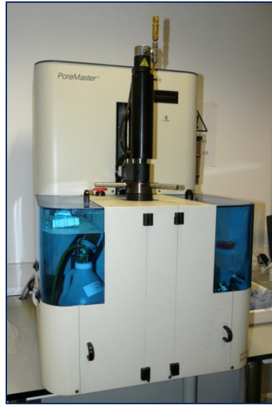
Figure 3-9. PoreMaster33 used for mortar porosity measurement
