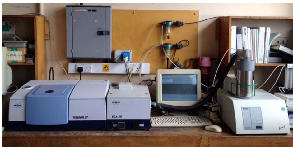
Figure 3-11. TG-FTIR instrument for \text{Ca}(\text{OH})_2 determination in fly ash/PC paste
