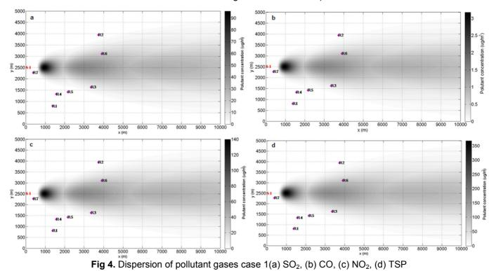
standard. Air pollutant dispersion from a single stack scenario and stack separated as far as 43 m showed much different results. The dispersion results for separated stack have tendencies for increasing the maximum concentration distribution and shorten the maximum concentration distance. This phenomenon was due to separated stack would produce lower flow rate pollutant.
