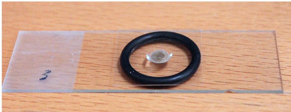
Figure A.2: Preparation of the hanging drop assay. A vacuum-greased O-ring is placed on a microscope slide, providing the support for a cover slide carrying a drop of sediment-containing water. The cover slide (thin squared glass) is placed upside-down, so that the drop is enclosed in the space sealed by the O-ring. Contact sealing by the vacuum grease prevents evaporation, preserving the drop for long observation under the microscope. Bacteria migrating towards the drop edge become visible under the optical microscope.
