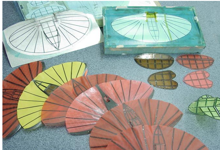
Fig. 5. Wing tools, tail sections, and fabricated wings.
