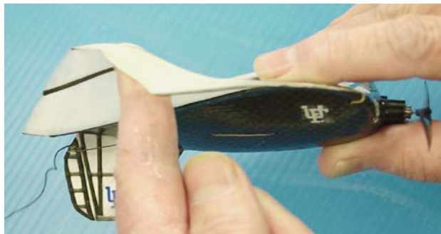
Fig. 3. The chord-wise compliance of a flexible wing allows for passive adaptive washout, increasing aircraft stability.
