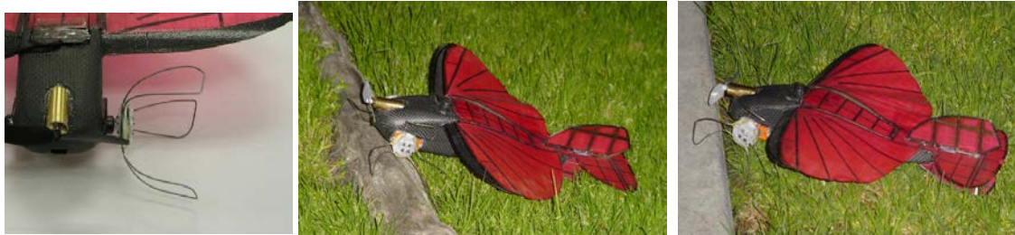
Fig. 8. MALV II has piano wire wheel-legs that are compliant on landing and resist becoming embedded in the substrate. These wheel-legs also enable it to crawl through grassy areas and climb obstacles taller than its leg length.
