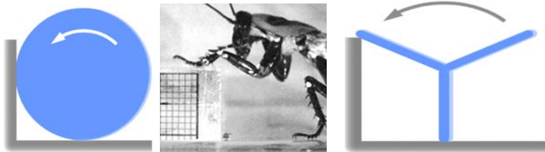
Fig. 1. The wheel-leg compromise between efficiency and ease of propulsion of a wheel and terrain mobility of legs.
