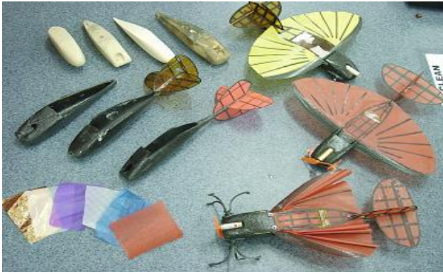
Fig. 6. Three completed vehicles, a series of fuselage tools, and an array of investigated wing fabrics. The bottom right vehicle shows a wing folding concept for future work.
