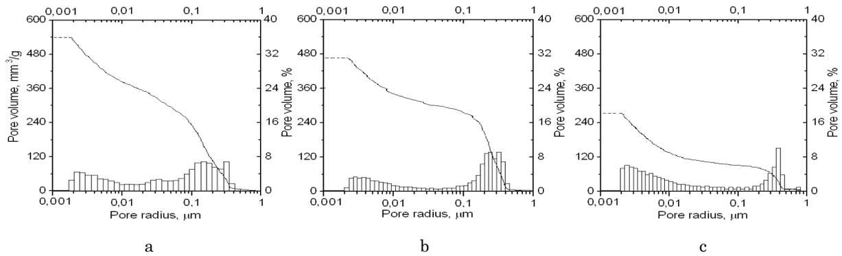
Fig. 1 – Pore size distributions of MgO-Al<sub>2</sub>O<sub>3</sub> ceramics sintered at 1200 °C (a), 1300 °C (b) and 1400 °C (c)
