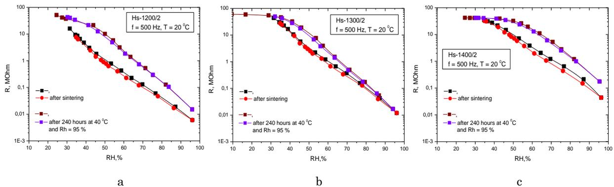
Fig. 2 – Exploitation properties of MgO-Al<sub>2</sub>O<sub>3</sub> ceramics sintered at 1200 °C (a), 1300 °C (b) and 1400 °C (c)
