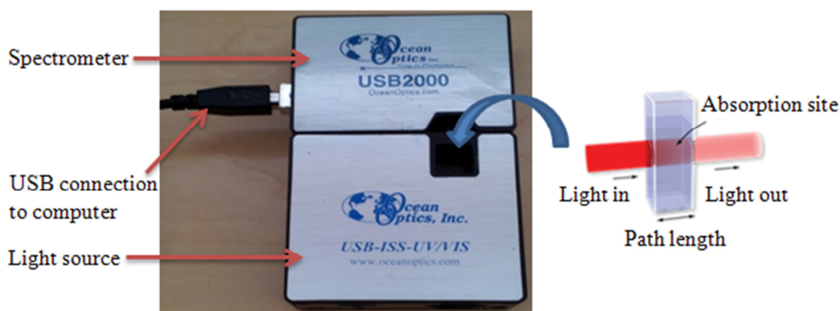
Figure 4.1: Typical setup of a Spectrometer with the light source and USB connections. A demonstration of a cuvette with experimental solution showing the absorption site and the location of cuvette placement for measuring absorption coefficients is also shown.
