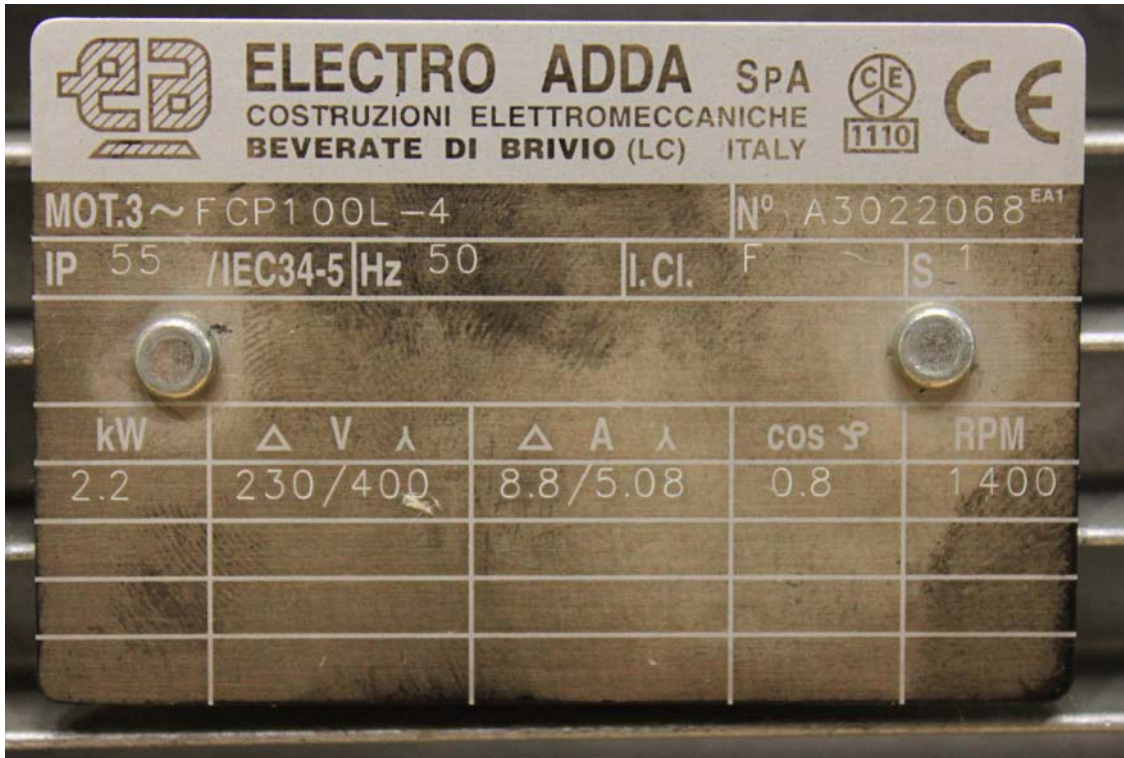
Fig. 3.27: A 2.2 kW induction motor nameplate
