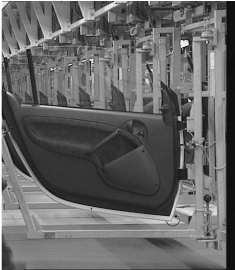
Figure 15.3. Detail of the left-hand-side door interior, showing fittings
