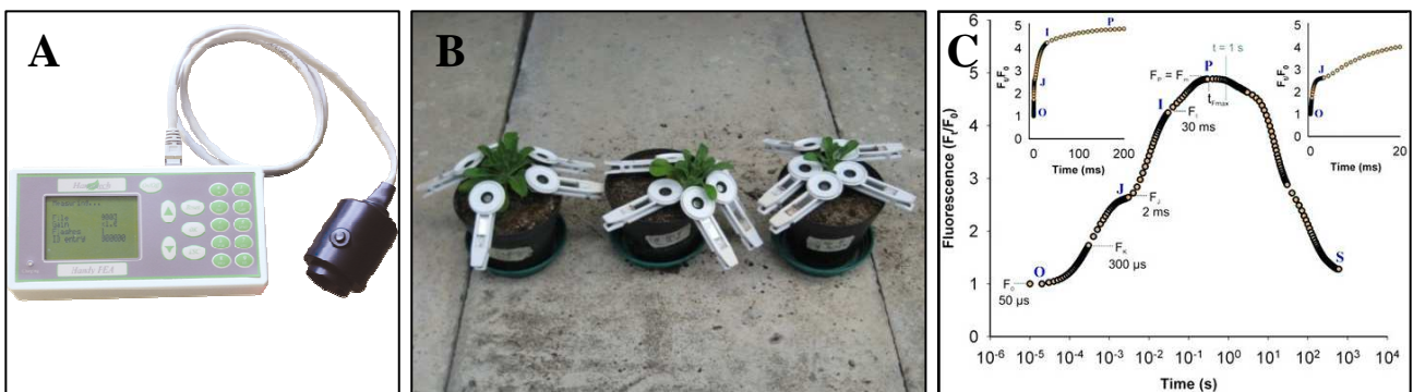
Figure 6. Fluorescence transient analysis. A) Handy-Pea fluorometer; B) dark adaptation of leaves samples as the first step of the chlorophyll fluorescence measurement; C) Kautsky Induction curve (Brestic & Zivcak, 2013) must be plotted on a logarithmic axis to observe the polyphasic rise to F_m .
