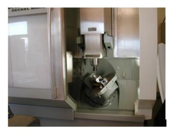
Figure 3.14: DMG 50 evolution 5-axis machining center
