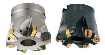
Figure 1.6: Face milling tools (Source: http://www.lmtfettetools.com)
