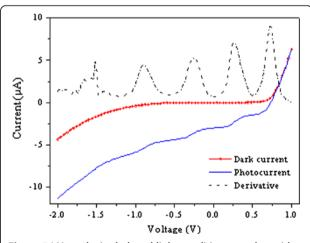
Figure 5 I-V results in dark and light condition, together with the derivative curves.
