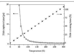
Figure 3 Temperature dependence of the hole  $\tau_{capture}$  (squares) and  $\tau_{cross}$  (stars) calculated for a 10-nm-thick QW.
