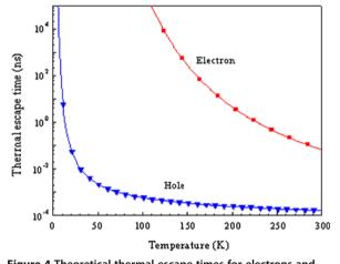
Figure 4 Theoretical thermal escape times for electrons and holes in the 10-nm-thick QW, as function of temperature.
