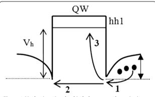
Figure 1 Mechanisms involved in hole capture dynamics into QW.
