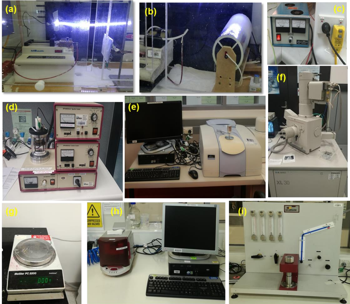
Figure 3-2: The equipment (a) electrospinning set-up with convex needle, (b) wire loop electrospinning, (c) high voltage power supply, (d) Sputter coating m/c, (e) FTIR, (f) SEM, (g) electric balance, (h) MMT tester, (i) Air permeability tester.
