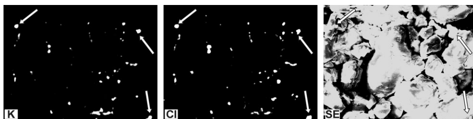
Figure 6. SEM image and EDS elemental maps of potassium and chlorine for the arrangement of KCl crystals within the glycine products containing 5000 ppm of additive. SE: SEM-EDS.
