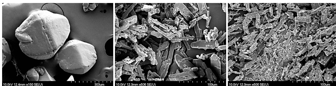
Fig. 3. SEM images of glycine crystals. (left: original crystal; middle: crystallized product A8; right: crystallized product B7).
