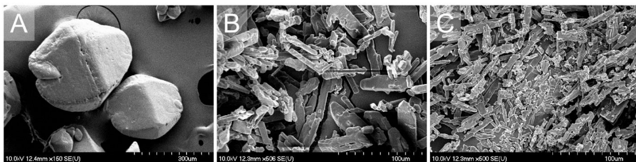
Figure 5 SEM images of the initial glycine (A); product of series A (B); product of series B (C).
