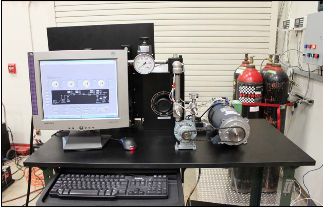
Figure 5.2-1: CAES Demonstration System Photograph
