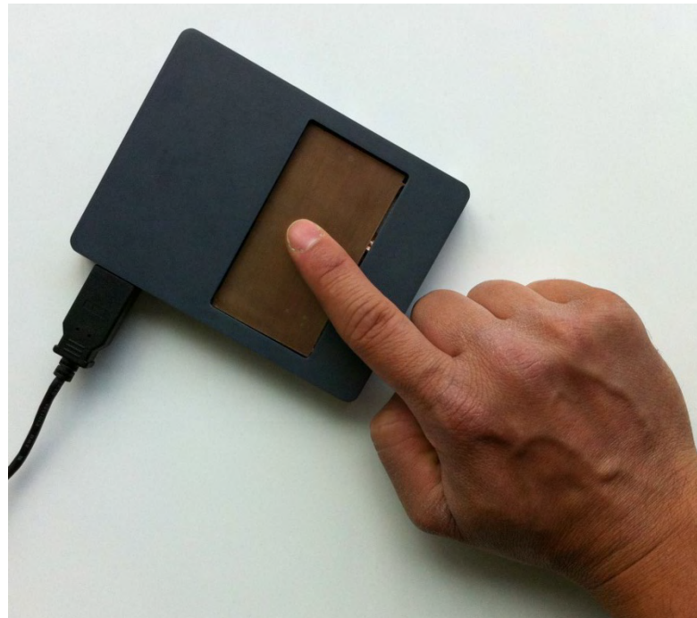
Figure VI.2: Photograph of the Stimtac prototype as presented in (Casiez et al., 2011). Reprinted with permission.
