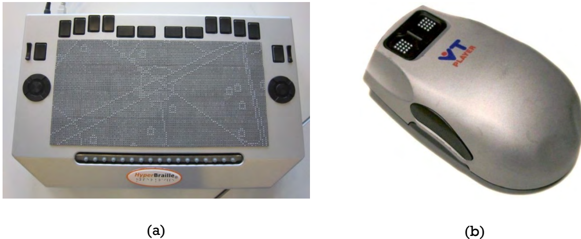
Figure II.13: Tactile actuator devices. (a) BrailleDis 9000 tablet as used by (Zeng & Weber, 2010). (b) VTPlayer mouse with two 4x4 arrays of pins. Reprinted with permission.
