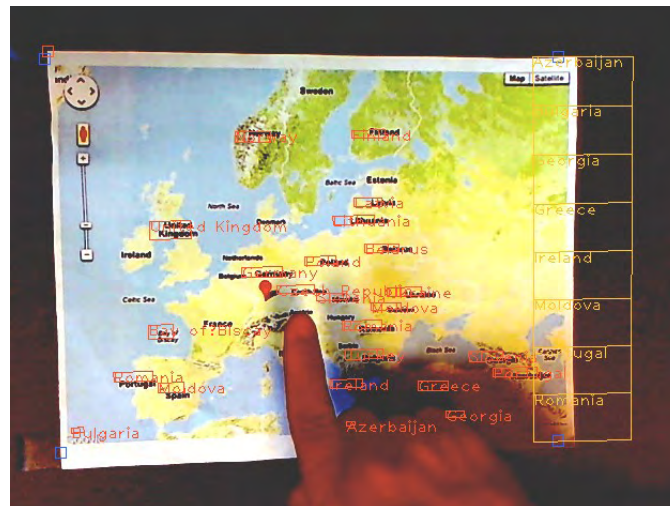
Figure II.15: Access Lens application as proposed by (Kane, Frey, et al., 2013). The map labels are located and recognized by image recognition and then translated into speech output. The menu on the right displays an index of on-screen items. Reprinted with permission.
