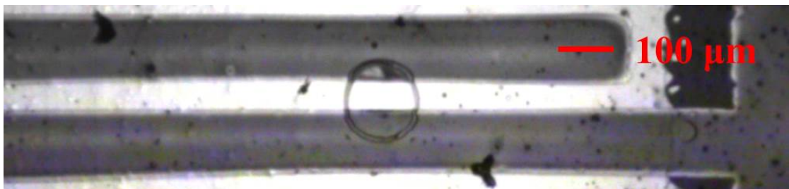
Figure 3.37: Single droplet printed on the channel of an OFET treated with FTP.
