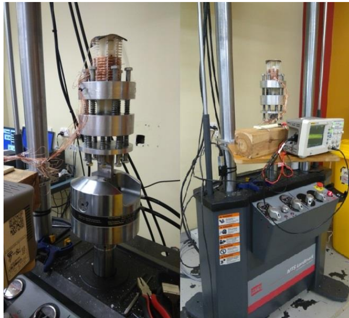
Figure 3.5: Experimental setup of the 2DOF electromagnetic vibration energy harvesting system on the MTS Landmark servo hydraulic test system (hydraulic shaker).
