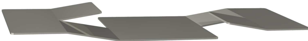
Figure 3.7.2: A schematic figure showing an electrode that has been shaped to act as a spring during first heating. The electrode has some spring force left even when pushed flat.
