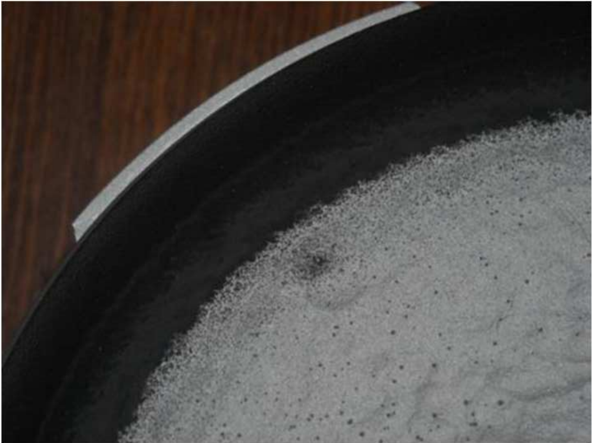
Fig. 3. Oxide nodules on used AlCr 70:30 at% cathode.
