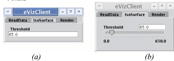
Figure 2: Two images showing the same tab of the user interface, (a) is using original (b) is generated from the extended skML
