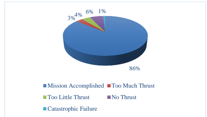
Fig. 6. Classification of failure scenarios for basic monopropellant design
