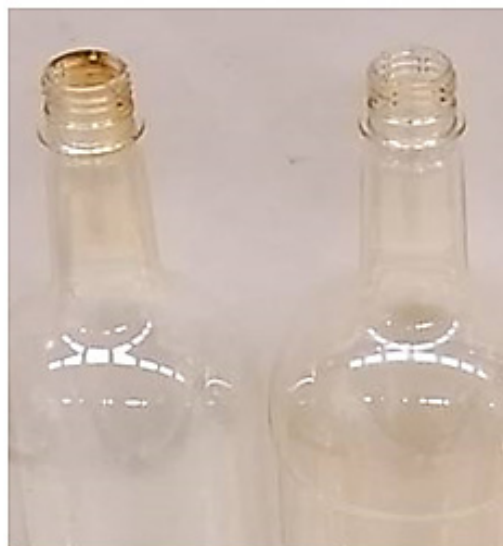
Fig. 7-2. An example of pre-commercialized DLC coated products for wine. The left was coated using conventional 13.56 MHz. The right bottle was coated using 6.00 MHz, and evenly distributed coating was achieved especially in mouth and neck parts, compared to the left bottle.
