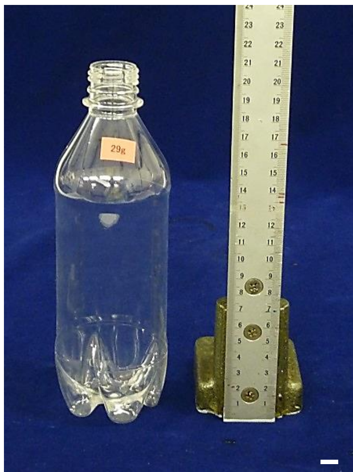
Fig.3-1. Appearance of PET bottles used. The shape of the bottle is typical for carbonated soft drinks. The bar represents 10 mm.
