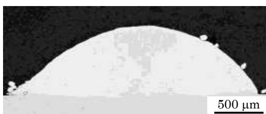
(a) Polishing surface with smearing
