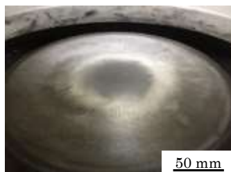
(b) Polishing paper causing smearing
