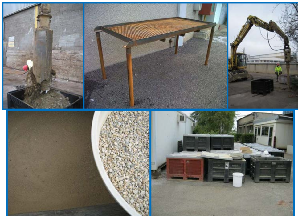
Figure II-2: Phase of soil sampling: drillings, prototype of screening table and storage.
