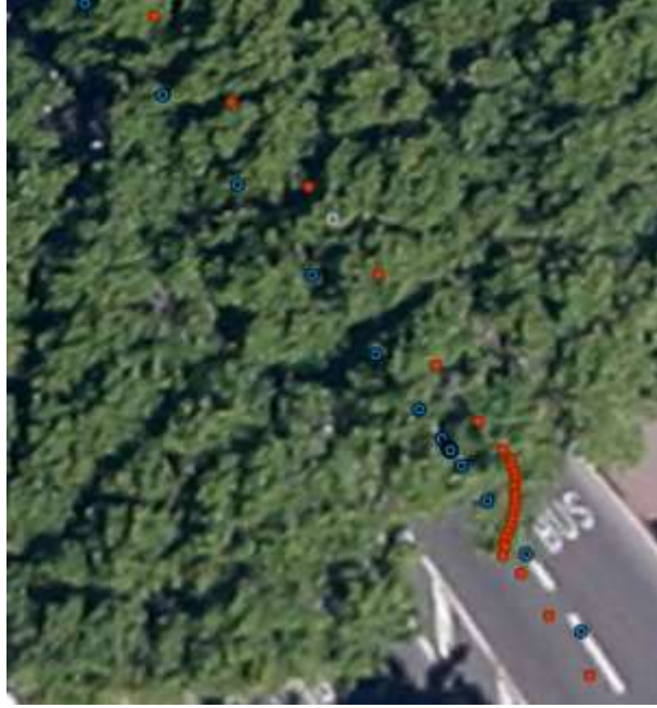
Figure 6.22 Example of drifting position due to high multipath during a static period, between hour 9.35 and hour 9.40. Orange spots indicate estimated position and blue spots indicate reference trajectory.
