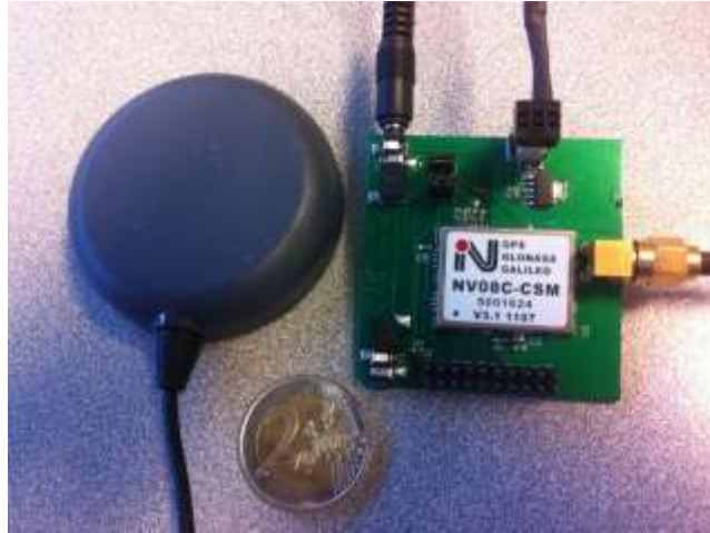
Figure 5.1 Receiver (on the left) and antenna (on the right) used in both data collections
