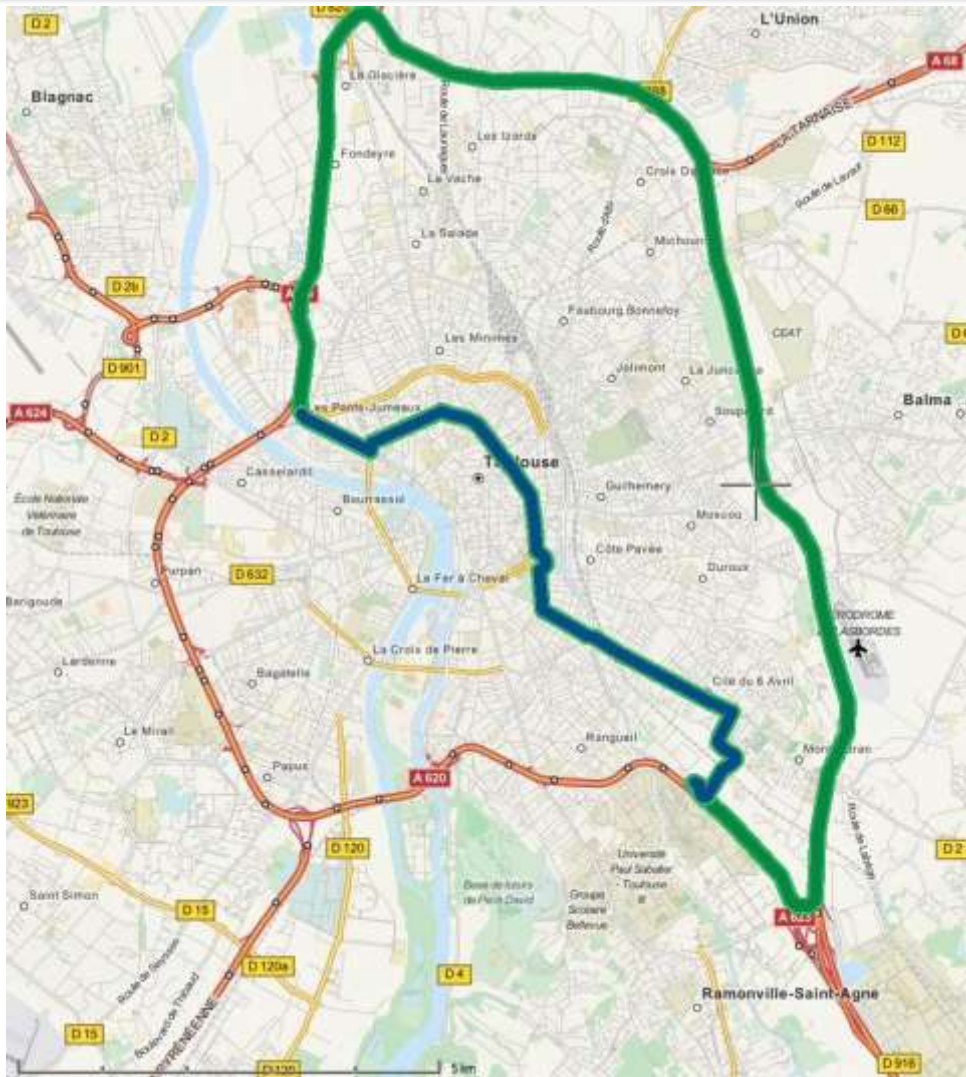
Figure 5.4 Test 1 trajectory. Urban environment is indicated in blue and beltway environment is indicated in green. Tiles Courtesy of MapQuest © OpenStreetMap contributors
