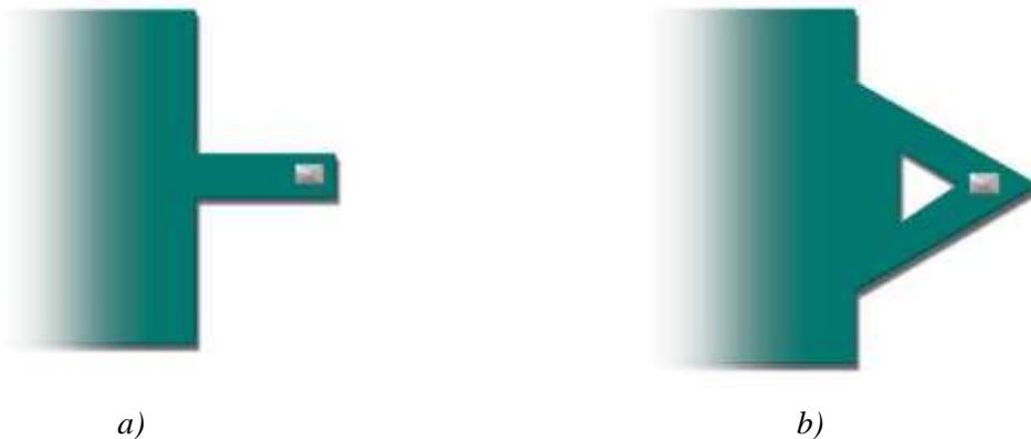
Figure 3.22: Schematic diagram of a) rectangular Non-Contact Mode cantilever and b) triangular Contact Mode cantilever
