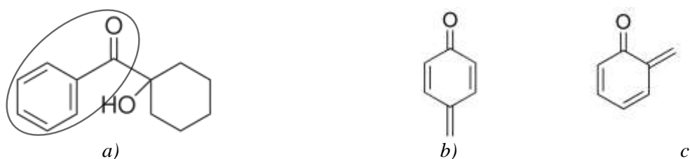
Figure 3.6: Chemical formula of HCPK photo-initiator (a) highlighting the phenyl group; the para (b) and ortho (c) orientation of the quinone methide
