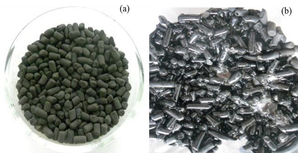
Figure 5.2 Photographs of coked catalysts from continuous process; (a) ZSM-5 particles from middle-bottom of PMMA cracking reactor (ZSM5-A) and (b) ZSM-5 particles from top of PMMA cracking reactor (ZSM5-B).
