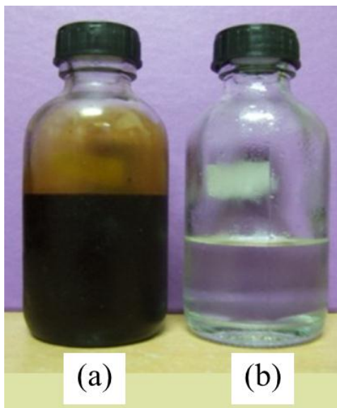
Figure 3.6 Liquid products from catalytic cracking of PMMA; (a) heavy fraction, (b) light fraction.
