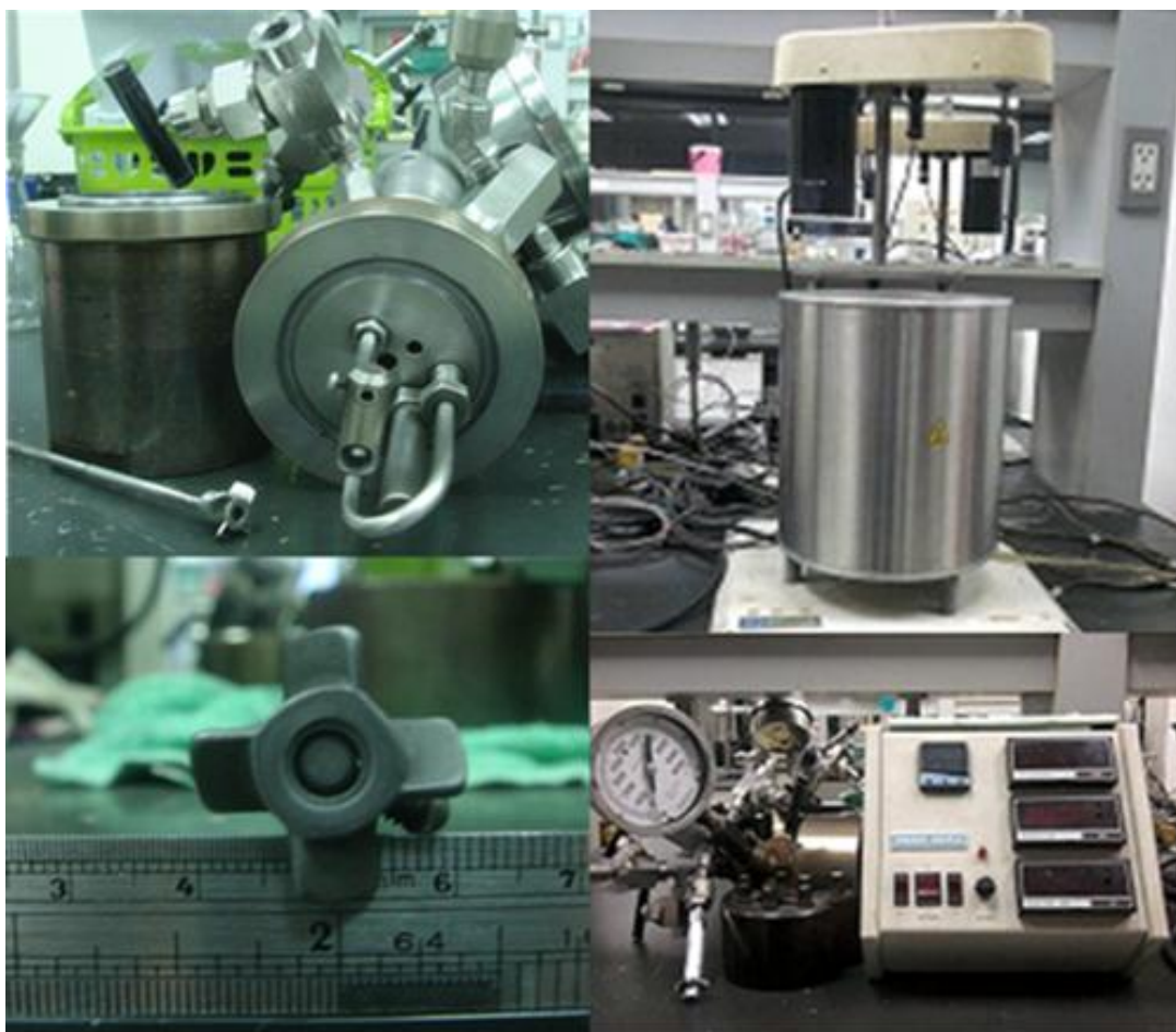
Figure 3.4 High Pressure/High Temperature Reactors 4576, 250 mL (Parr instrument).
