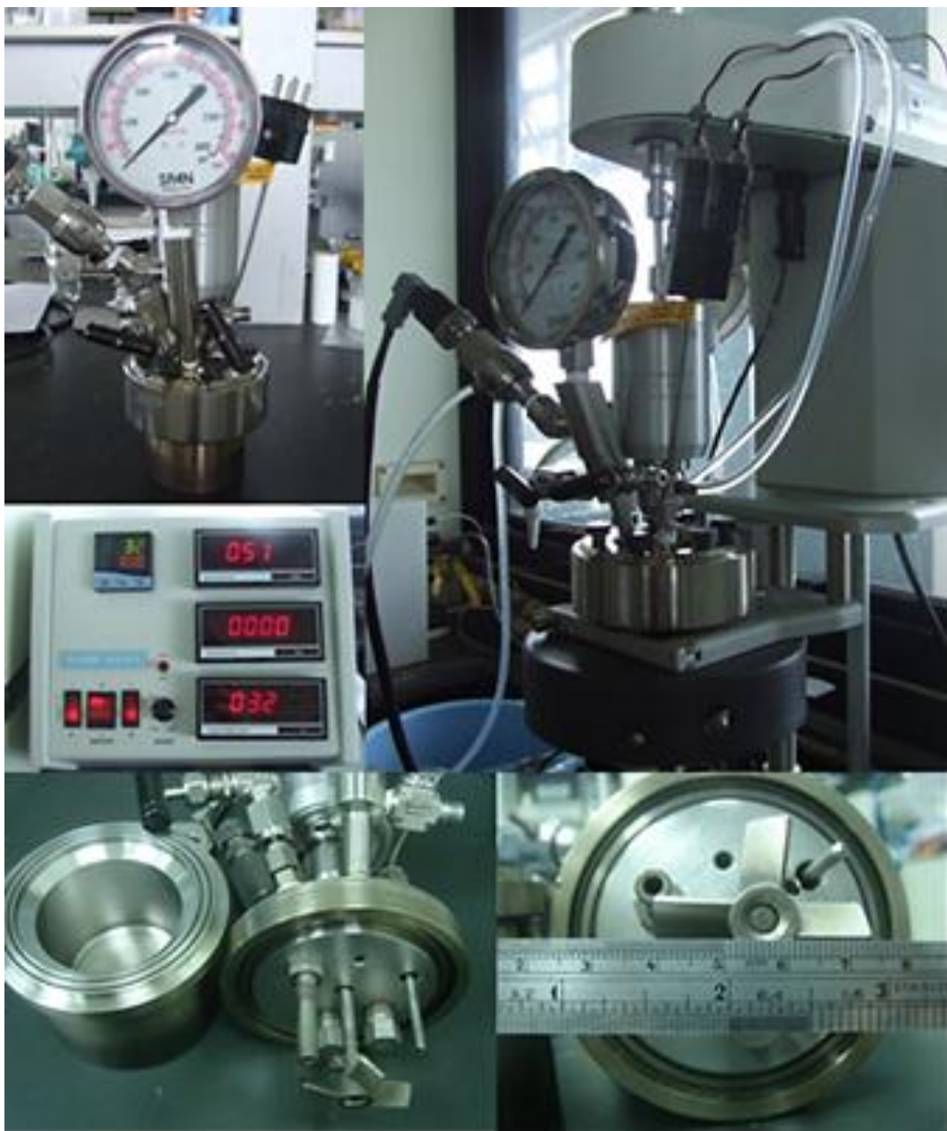
Figure 3.10 Mini bench top reactor 4560, 100 mL (Parr instrument).
