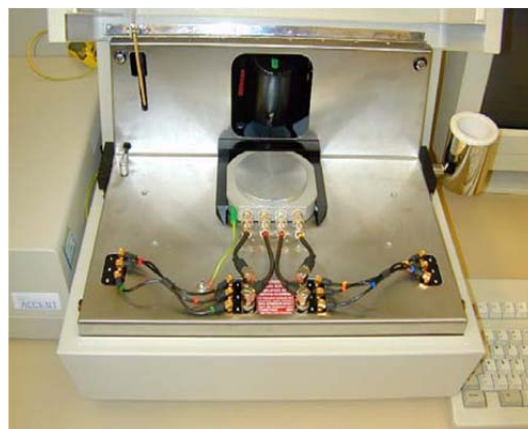
Figure 63: HL5500PC Hall Effect Measurement System.
