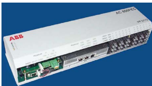
Figure 54, ABB's AC 800PEC, core of the OPCoDe system
