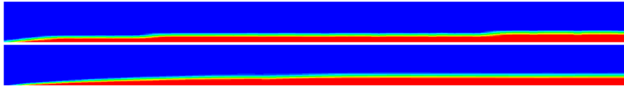
Figure II.8 – Alignment of the interface on the mesh when VOF scheme is too compressive, for example with the Geo-Reconstruct scheme (top) compared with the HRIC scheme (bottom)
