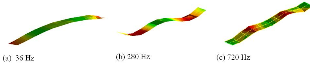
Figure IV.15. Vibration modes of the CFB.
