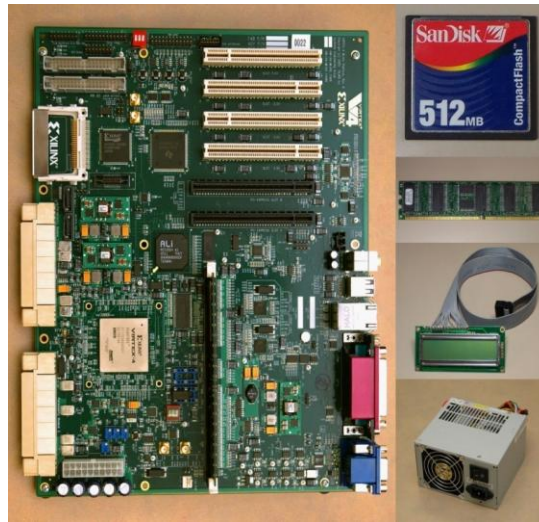
Figure II.26 La plateforme ML410 FPGA-Xilinx.
