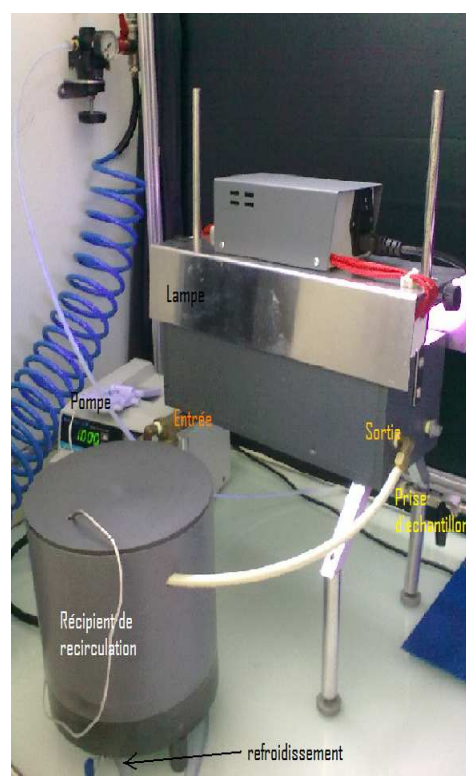
Fig. II -11. Schematic representation and photography of the channel reactor
