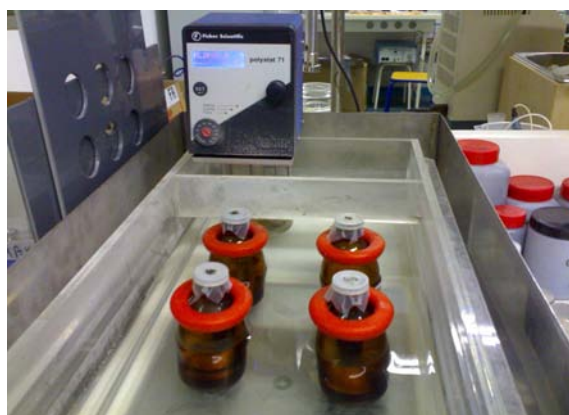
Fig.II-10. Static multifunction thermostatic bath used for the adsorption isotherm.
