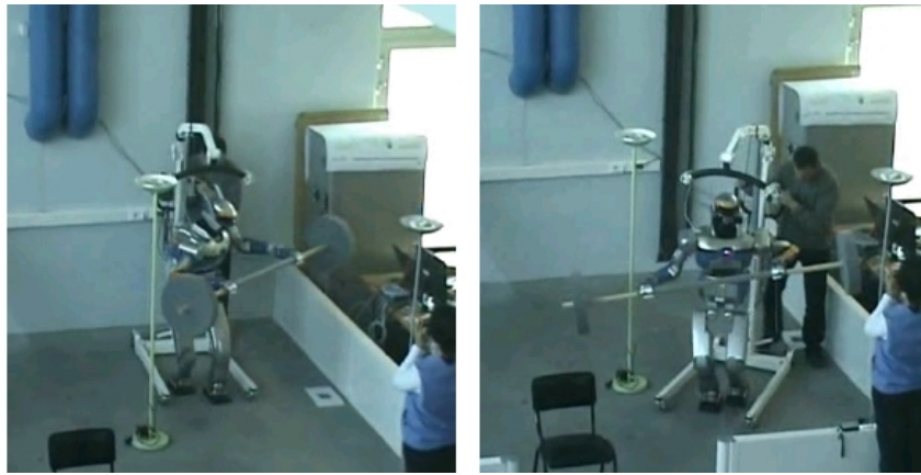
Figure 1.7: From [Esteves Jaramillo 2007]: the robot HRP-2 is carrying an object from one place to another while avoiding collisions between its own body, the manipulated object and the other objects in the environment.
