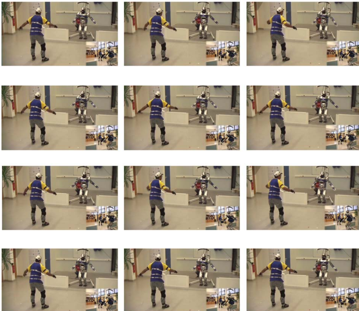
Figure 4.14: Dancing motion: in this sequence the motion include movement on the head, chest, arms and waist. Here, the kalman filter is very important because arms hidde some markers to the system. Its position is estimated by the filter.
