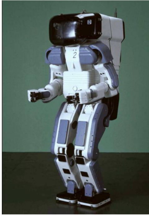
Figure 1.5: P2: the Honda humanoid presented in 1996 that was capable of walking and climbing/descending of stairs. It is 210 kg weight and 182 cm height. Picture source http://asimo.honda.com
