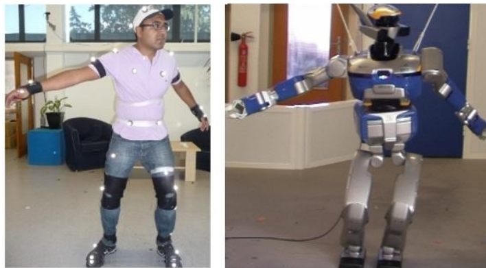
Figure 4.3: Scenario 1: snapshot of human dancing and its imitation by HRP2.
