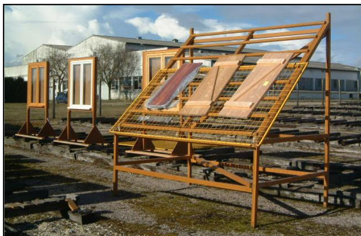
Figure 4.35 Natural ageing device with Wood Protect® window shutters
