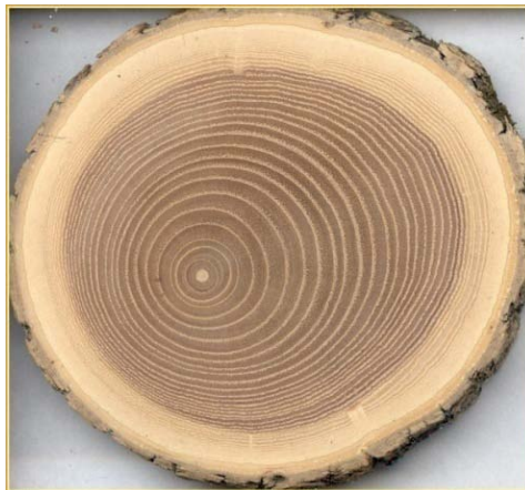
Figure 1.4 A section of a trunk showing the annual growth rings, pale sapwood and dark heartwood, and pith 10
