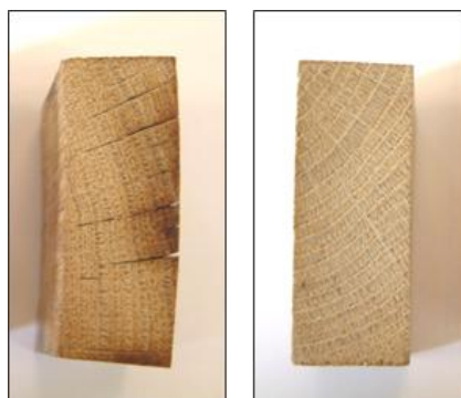
Figure 4.34 Samples of oak after ageing in weathering chamber
