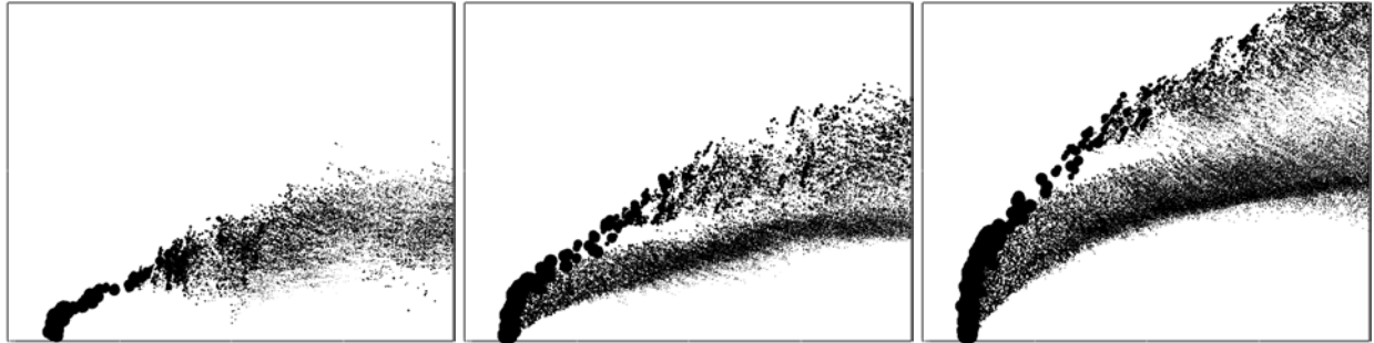
Figure 6.28 : Closeup view of the column and of the atomizing spray. From left to right: q = 2, q = 6, q = 18
