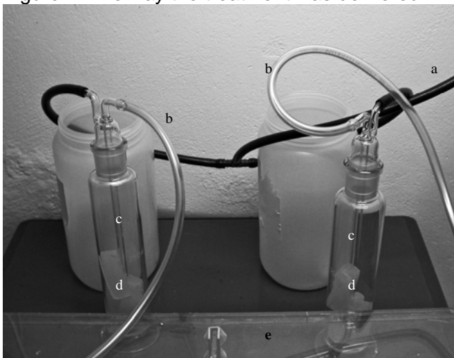
a: pipe driving the air from the gas bottle to the bottle containing the treatment ; b: pipe leading the air charged with the treatment to the test box ; c: bottle containing the treatment; d: the blocks (treatment and control) are divided in pieces ; e: test box.
