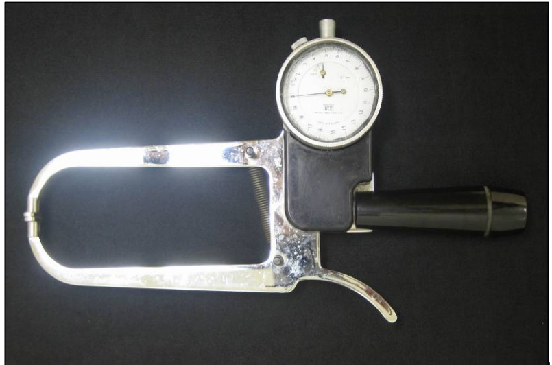
Figure 3. Calipers, tool for the diameter and deformability.
