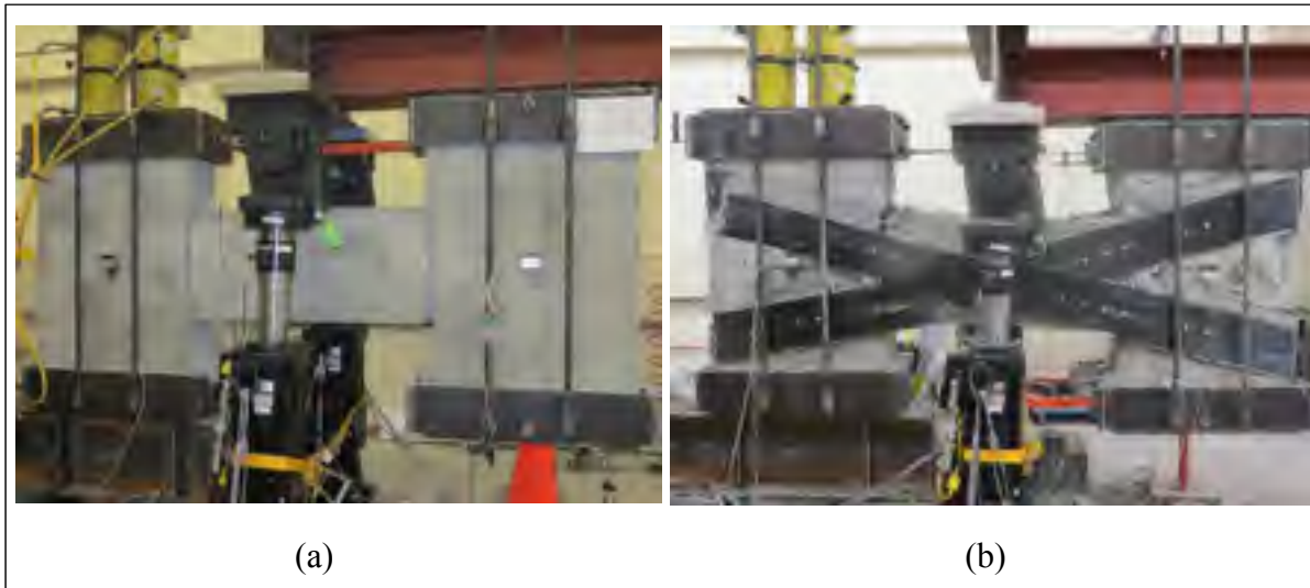
Figure 4.7 Crack pattern of specimens at failure: (a) CB.CONV, (b) CB.CONV-R
