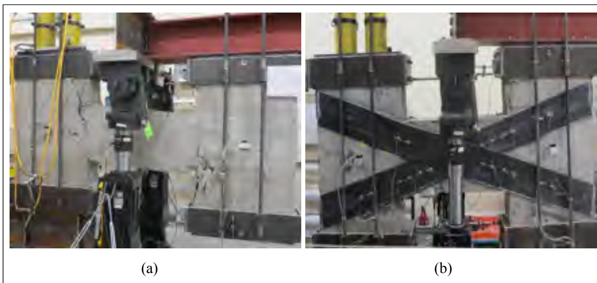
Figure 5.5 Crack pattern of specimens at failure: (a) CB.DIAG, (b) CB.DIAG-R
