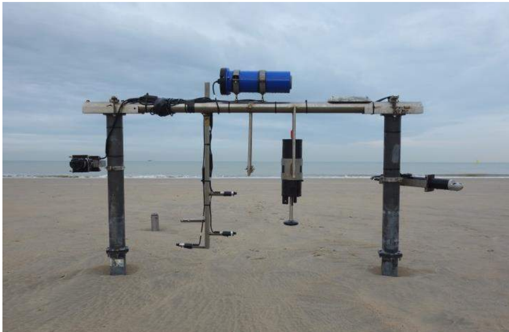
Figure 1. Intertidal measuring frame with 3 optical backscatter sensors, 3 acoustic current profilers, 1 electromagnetic current meter, and 1 pressure sensor (not on photograph).
