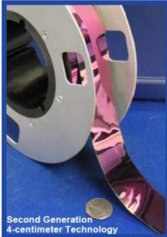
Figure 4.4. Actual 2nd Generation YBCO tape from American Superconductor with a tape width of 4 cm and a thickness of 0.21-0.23 mm.
