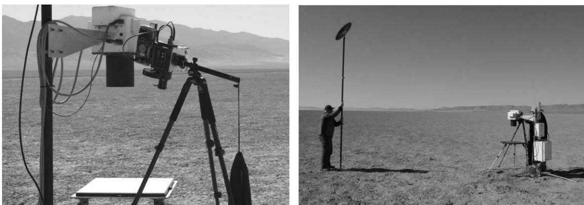
Figure 6. CaTSSITTR and GVR viewing white reference as part of an SRBC collection at Railroad Valley Playa, Nevada. Right hand photo shows shading of the reference to provide measurement of diffuse skylight irradiance.
