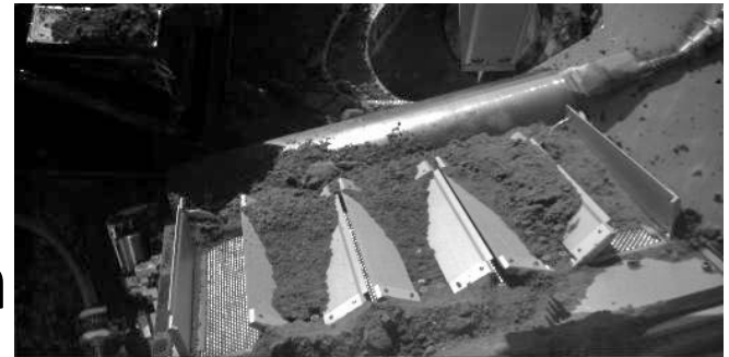
Phoenix sample bin door faults. Bonitz et al. 2008
