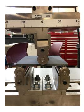
Figure 8: Setup of for three point bending
