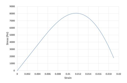
Figure 11: Shear stress versus shear strain used to obtain functional degradation of shear modulus  $\mathcal{G}_{12}$
