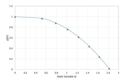
Figure 17: State variable  $S_r$  vs g used to represent degraded shear modulus  $G_{12}$  for the third method
