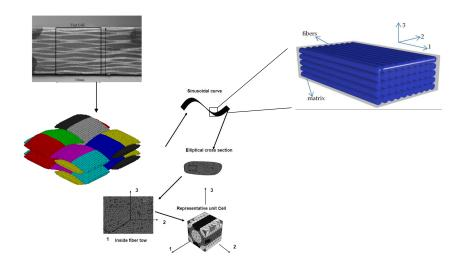
Figure 1: Hierarchical structures of textile composites.
