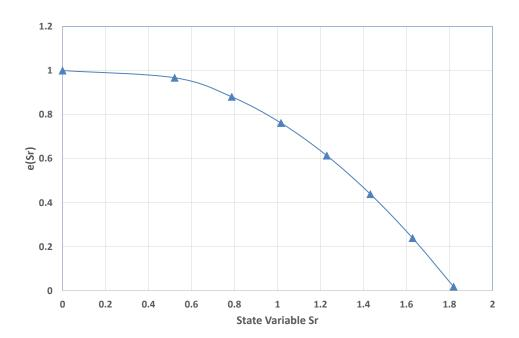
Figure 16: State variable  $S_r$  vs e used to represent degraded transverse Young's modulus  $E_2$  for the third method
