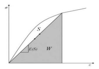
Figure 2: Schematic of state variable  ${\cal S}$  and recoverable energy density  ${\cal W}$  [6]
