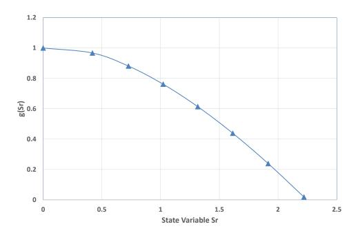
Figure 15: State variable  $S_r$  vs g used to represent degraded shear modulus  $G_{12}$  for the second method
