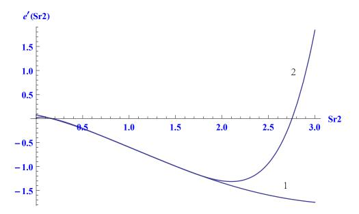
Figure 21: Comparison of derivative of internal state variable for two formulation. The curve 1 is from the derivative of Eq (32) and the curve 2 is from the derivative of Eq (34)
