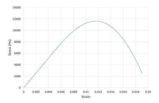
Figure 10: Transverse stress versus transverse strain curve used to obtain functional degradation of transverse Young's modulus  ${\cal E}_2$
