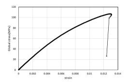
Figure 5: Stress strain curve for shear modulus
