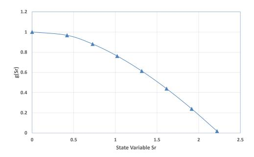
Figure 13: State variable  $S_r$  vs g used to represent degraded shear modulus  $G_{12}$  for the first method
