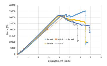
Figure 9: Comparison of simulations with test data of three point bending
