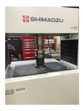
Figure 3: Setup of compression test
