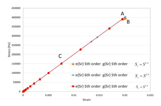
Figure 19: Comparison of simulations of notched square panel under compression for three methods. All three methods produce similar results, indicating objectivity of the microdamage evolution equation with respect the functional form of the microdamage functions.
