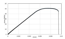
Figure 4: Stress strain curve for transverse modulus
