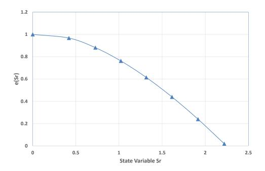
Figure 14: State variable  $S_r$  vs e used to represent degraded transverse Young's modulus  $E_2$  for the second method
