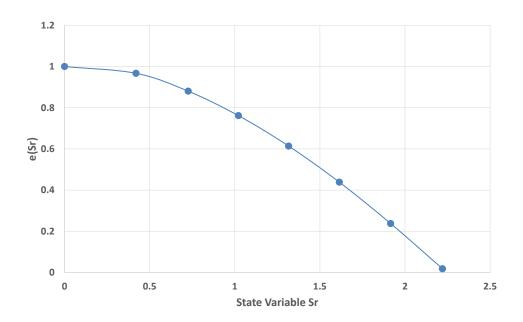
Figure 12: State variable  $S_r$  vs e used to represent degraded transverse Young's modulus  $E_2$  for the first method
