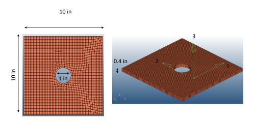
Figure 18: Finite element model of 10 in. by 10 in. by 0.4 in. notched panel
