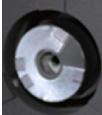
Figure 4.—Mo mask on keeper electrode.
