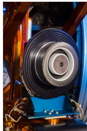
Figure 3.—TDU-1 in VF-6 configured for short-duration wear testing.
