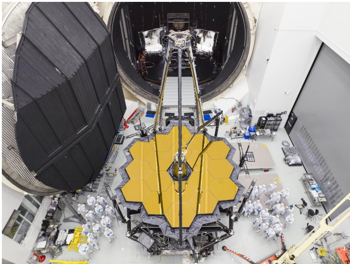
Figure 23. The OTIS, in the cleanroom outside of JSC's historic Chamber A, after its successful cryo-vacuum test campaign.
