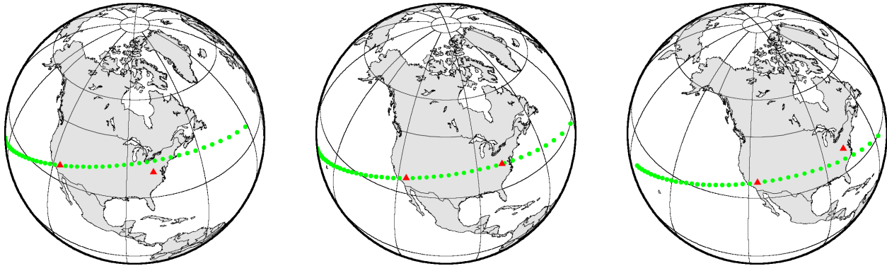
Figure 2. Radar echoes from Mercury sweep over the surface of the Earth. Diagrams show the trajectory of the speckles one hour before (left), during (center), and one hour after (right) the epoch of maximum correlation. Echoes from two receive stations (red triangles) exhibit a strong correlation when the antennas are suitably aligned with the trajectory of the speckles (green dots shown with a 1-s time interval). From Margot et al. (2012).
