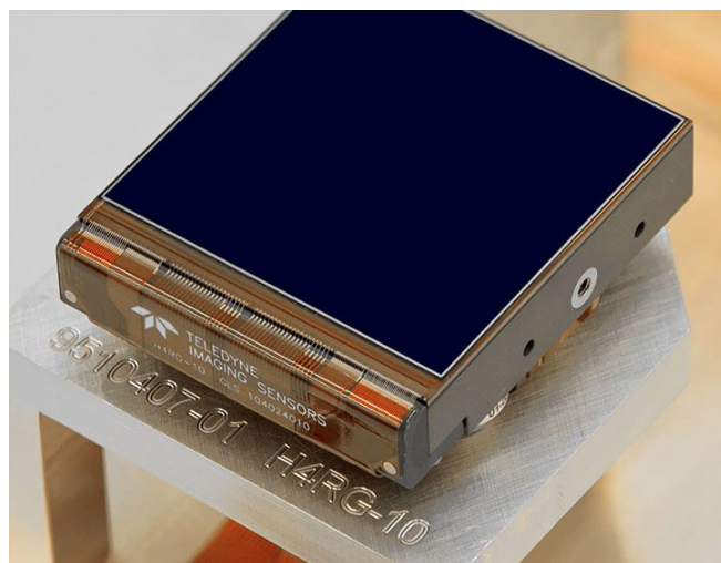
Figure 3. Left: Image of H4RG array from Teledyne website. Right: Cartoon of HgCdTe array on silicon multiplexer from Ref. 9.
