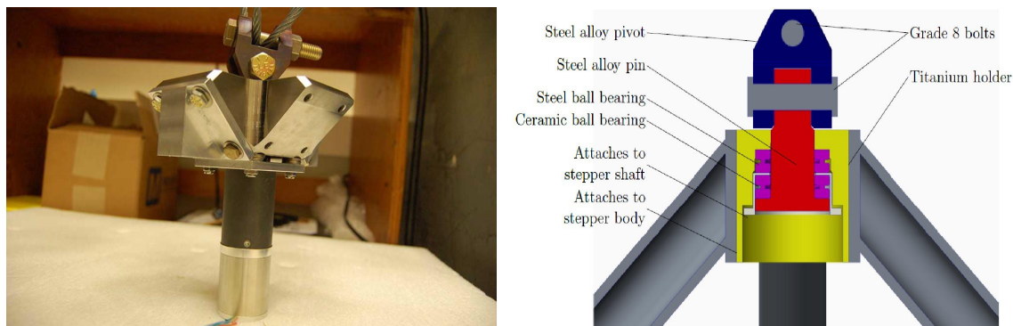
Figure 7: The pin that attaches to the balloon contains the stepper motor and the bearings to dump momentum to the balloon attachment assembly
